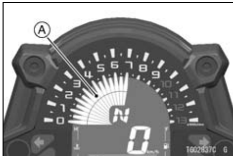
A. Shift-up Indicator (Tachometer Gauge)
